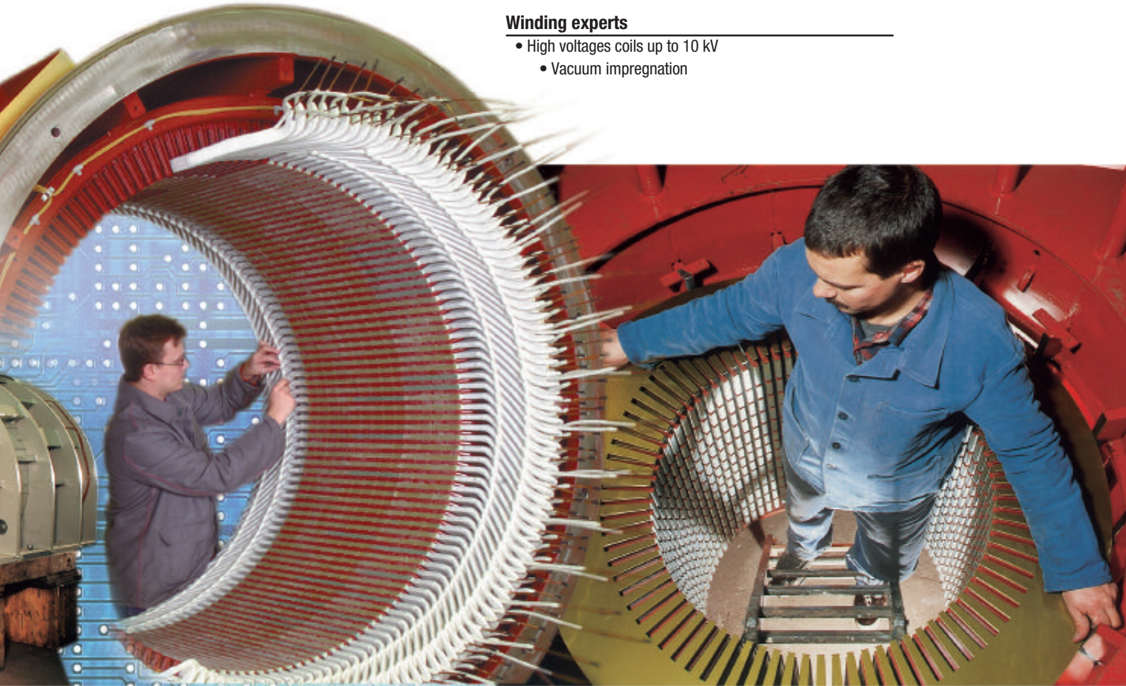
Installation and connection of coil
