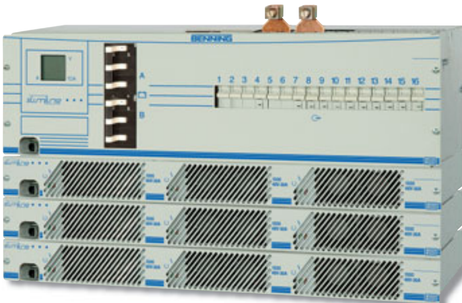
Fig. 11: Rectifier, Distribution SMS 13500: 2 x Battery breaker 9 x 48 V – 1500 W 16 x Load fuses
